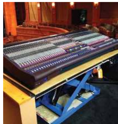
The Midas Heritage 3000 house console on a hydraulic platform so it can be quickly lowered and retracted under the walls.
